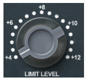
Maximum level allowed by the limiter on the plugin output. 0.5 dB steps.
