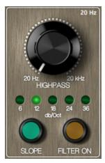
Filter that blocks the lower frequencies of the signal.
